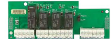
WS4-EXT, extender that can be added to the WS4-1D-E electronic to convert it into the WS4-2D-E (electronic for the 2 door webserver controller)
