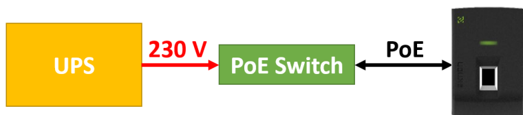
Obr. 5: PoE switch s UPS
